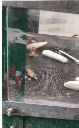
Figure 3. The grasshopper maquette and dead and alive grasshopper that placed in wind tunnel during the test
