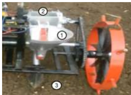
Figure 4 and 5- Position of designed and developed seedling distributor and seed storage and (1: seed storage)
