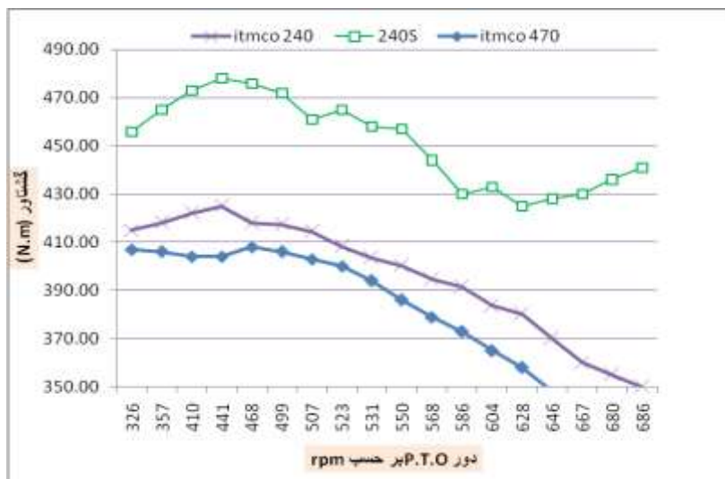
Figure 2. Comparison of the torque of the studied tractors
