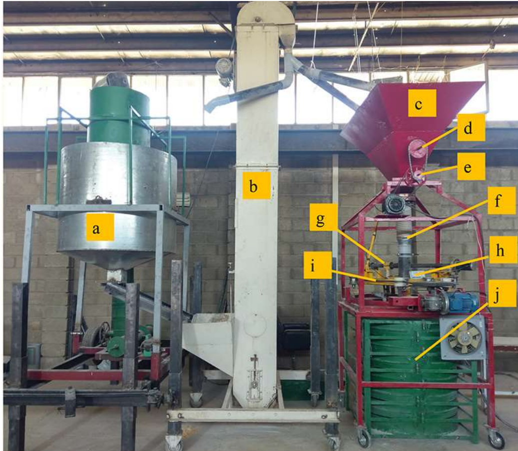
Fig. 2. Experimental set up (a) main container, (b) elevator, (c) trapezoidal container, (d) agitator, (e) fluted roller mechanism, (f) fill pipe, (g) reciprocating mechanism, (h) unit control system, (i) rotating rim (j) pilot scale silo consist of seven rings
