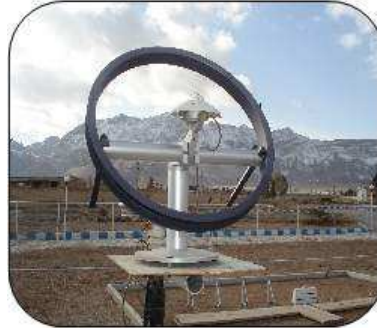
Figure1- Pyranometer for measuring radiation energy
