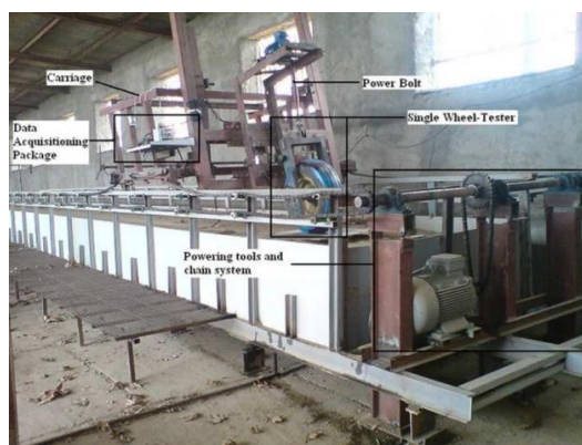
Figure 1- Soil bin system set up and including carriage and a single wheel-tester
