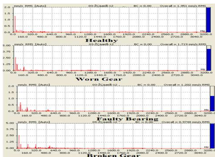
Figure 2-Vibration signals of MF-240 Tractor gearbox in different states.
