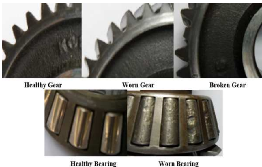
Figure 1- Gearbox faults
