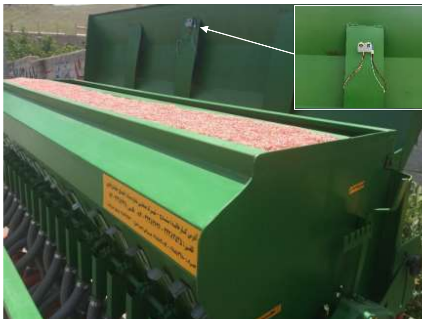
Figure 4. Implementation of the ultrasonic level meter system on a grain drill.
