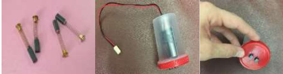
Figure 9. Graphite probe made with a pair of carbon brushes
