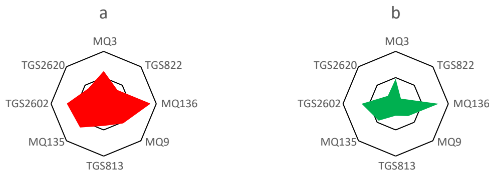
Figure 2. Radar graph response of the sensors for Fresh chicken (a), Frozen chicken (b).
