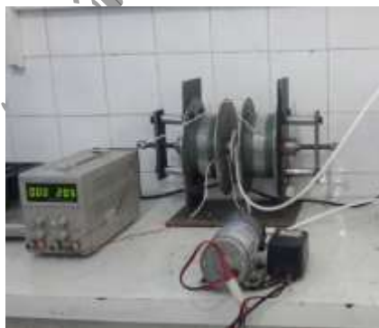
Figure 1. Magnetic Water Supply and Power Supply.
