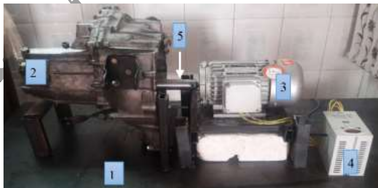
Figure 3. The components of the monitoring system, 1- Desk 2- Gearbox 3- Electromotor 4- Inverter 5- Shaft
