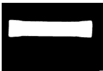
Figure 3. The final image of one of the tines for determining the surface area
