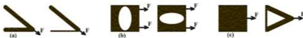
Figure 5. Different types of optimization categories: size (a), shape (b) and topology (c).
