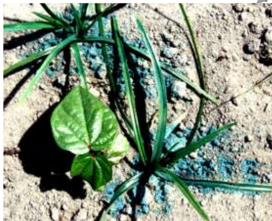
Figure 2. Field test of robotic weed control system equipped with a precision micro-sprayer showing blue dye selectively applied to nutsedge ( Cyperus spp.) weeds in a cotton field (Lamm et al., 2002).
