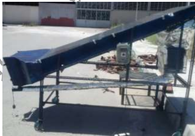
Figure 1. View of the solar dryer with collector plate, cabinet, recycling heat exchanger
