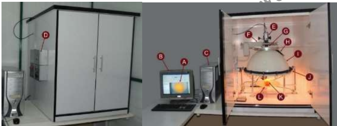
Figure 1. The Vis-NIR spectral imaging system; a. Online image of sample, b. Computer monitor, c. Computer, d. Control panels of lighting system and motors of displacement, e. Vis-NIR camera, f. Guidance system for changing the filters, g. Placement of the filters, h. Cooling fan, i. Aluminum hemisphere of lighting system, j. Light-dispersing illumination system, k. Sample for imaging, l. Plate of sample placement.
