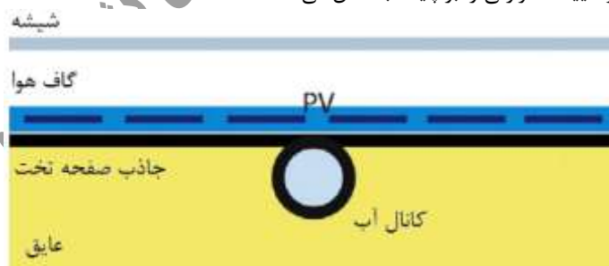
Figure 1. Schematic of water based photovoltaic-thermal system
