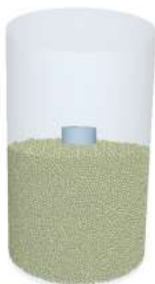
Figure 3. Discrete element model of plate sinkage in soil.
