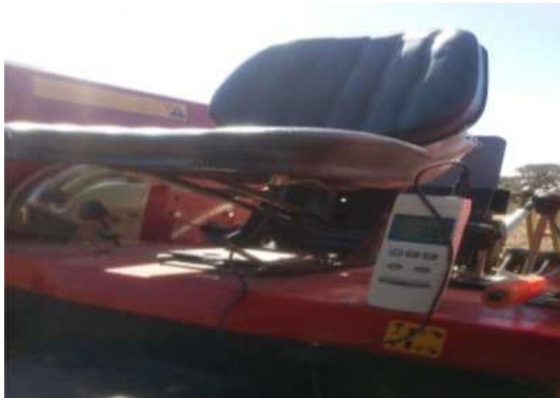
Figure 3: How to connect the vibration meter to the driver's seat
