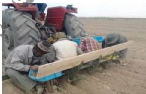
Figure 3- Transplanter without conveying mechanism equipped with moldboard furrowers
