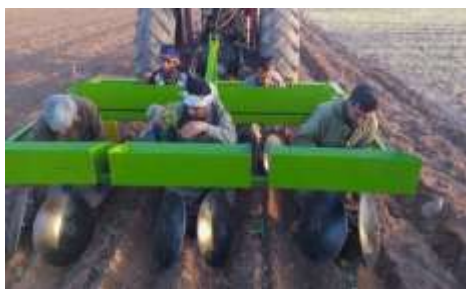
Figure 2- Transplanter without conveying mechanism equipped with disk ridgers
