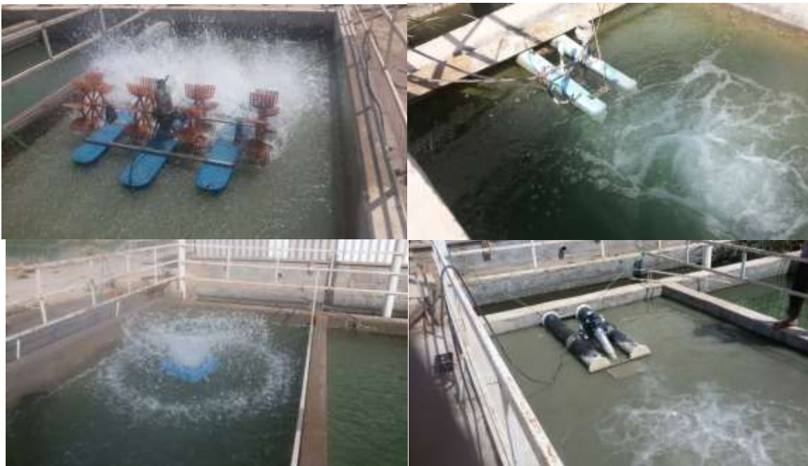
Figure 1. The aerators used in the experiment: Up from right to left: circulator and paddle wheel aerators and down from right to left: Propeller-aspirator and vertical aerators
