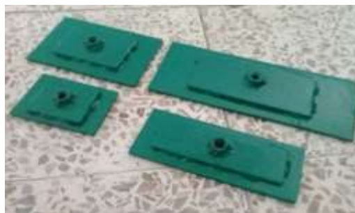
Figure 2. View of the Bekker pages installed on the device probe.
