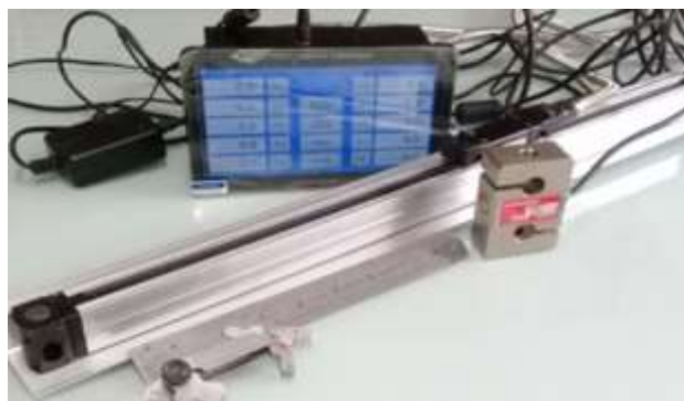
Figure 3. Digital ruler, data logger and load cell used on the device.
