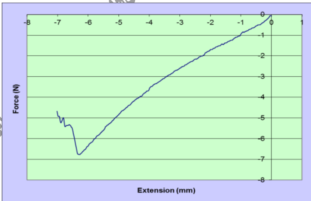
Figure 3. Force versus extension variations for Cherry tomato
