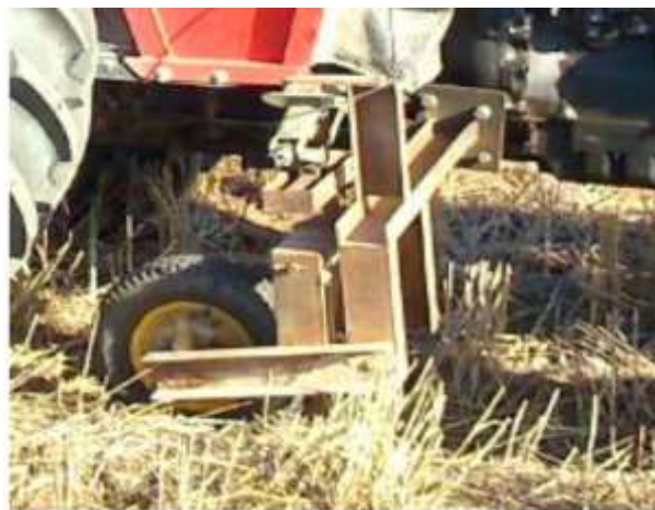
Figure 2 . The fifth wheel used to measure the actual speed of the tractor
