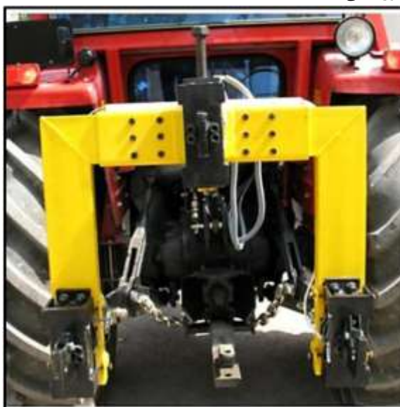
Figure 1. Three-point connecting dynamometer used in this research
