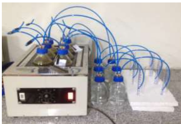
Figure 1: Measurement of biogas by water displacement method (Drosg 2013).
