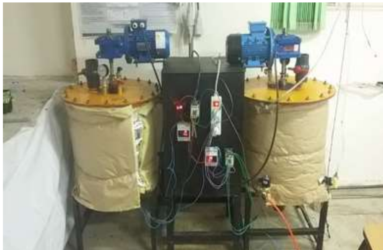
Figure 2: Reactors made to produce biogas
