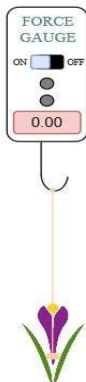
Figure 3. Measuring the force of separating the saffron flower by force gauge.
