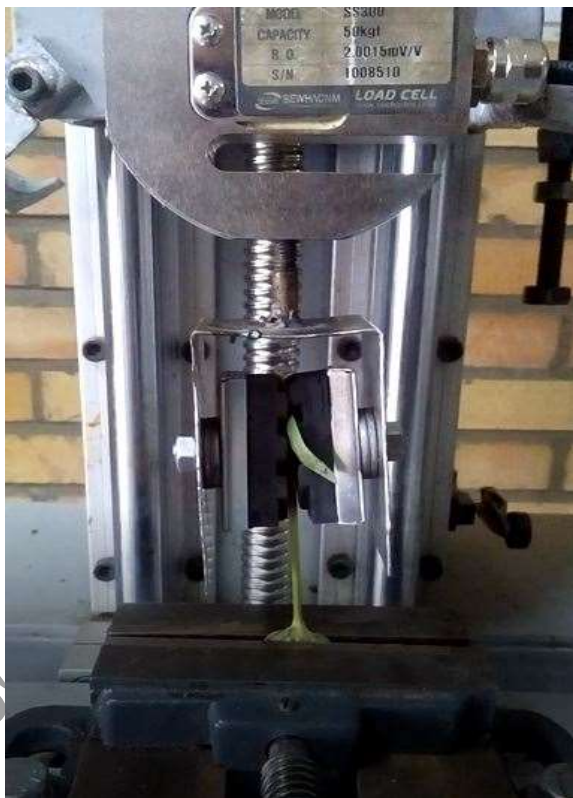
Figure 4. Controlling the sample by special clips
