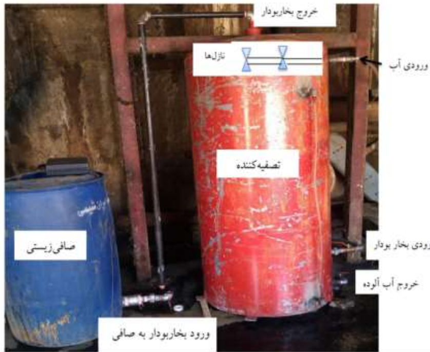
Figure 5. The pilot system that constructed for odor control system.
