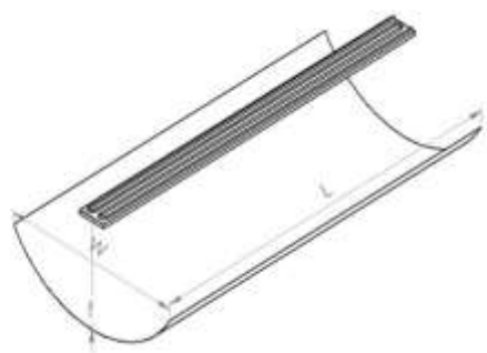
Figure 1. Schematic of a Parabolic Linear Concentrator with PV Photovoltaics
