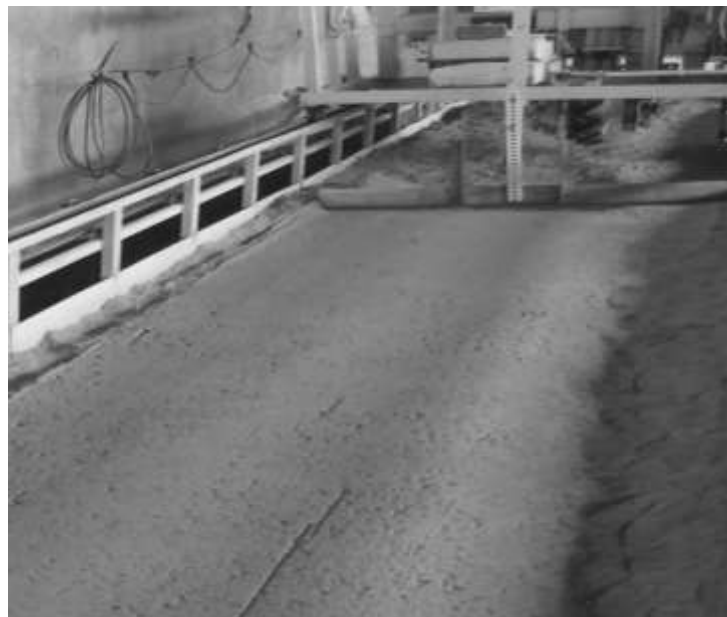
Figure 1. The process of soil bin surface leveling
