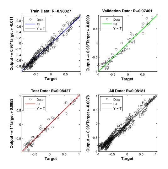
Fig. 2. Regression result of developed ANN for TFC parameter using Levenberg-Marquardt training algorithm.
