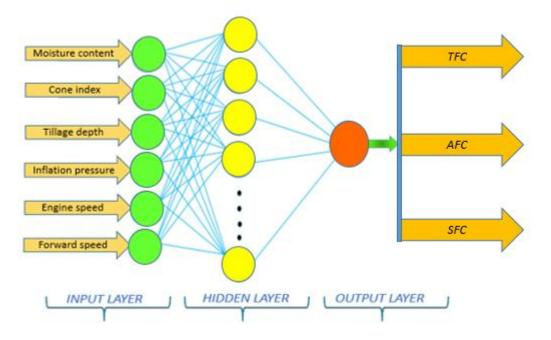
Fig. 1. Schematic architecture of the used ANN
